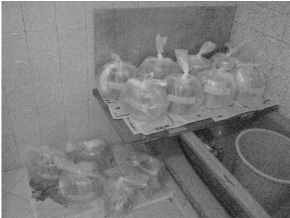
Fig. 4. Curing room for CBR samples
